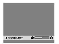
\* If neither the destrip or button is pressed within 5 seconds, the current setting is set and the previous screen reappears. 4. Press the "PROCEED" button. The contrast adjustment is completed.
